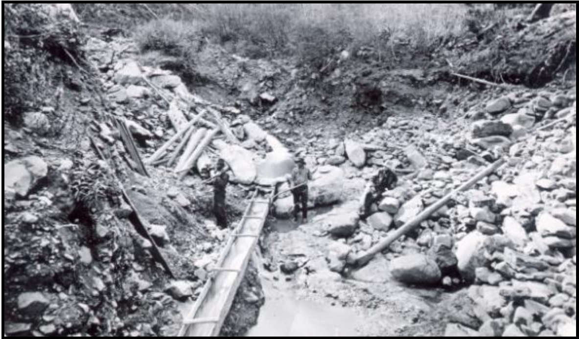
Illustration B 1.1: The photo depicts a typical gulch placer mine, featuring a sluice on one side of the drainage floor, tailings on the other, and high-bank excavations on both sides. Although the mine is in La Plata County during the mid-1870s, the general form was universal. Courtesy of Denver Public Library, WHJ-10197.
